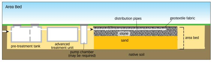
A side view of an area bed following an advanced treatment unit. Note: some system designs allow for the treatment unit to be located on top of the area bed.
