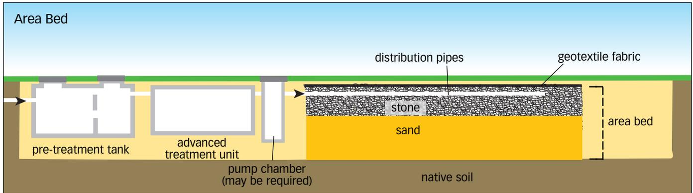
A side view of an area bed following an advanced treatment unit. Note: some system designs allow for the treatment unit to be located on top of the area bed.
