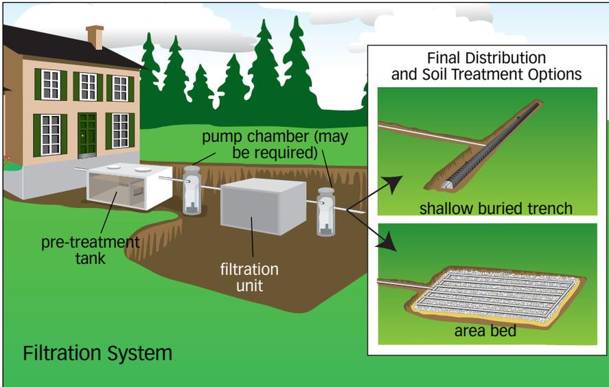
Effluent from a filtration unit can be distributed back into the native soil through a shallow buried trench or an area bed.
